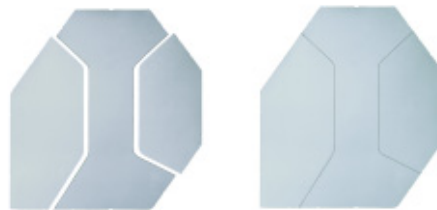
Individual parts of an engineered blank before and after welding.
